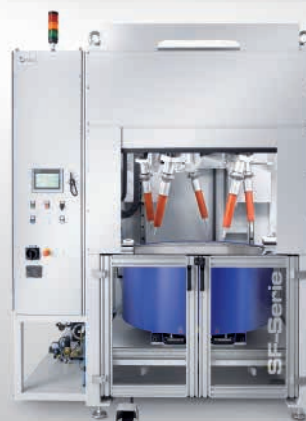
OTEC SF Stream finishing machine
