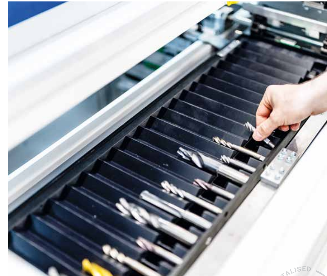
Prism-grooved pallets with unsorted tools
