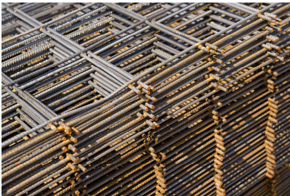
Reinforcement mesh produced by forming rollers
