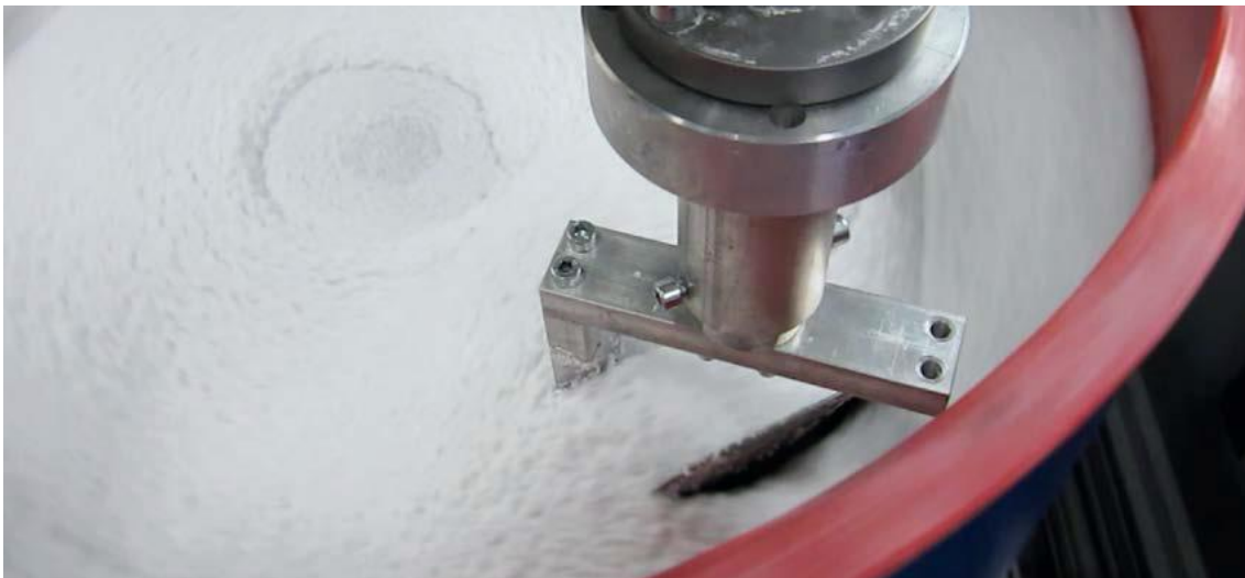
Clamping assembly of the turbine blade during the process
