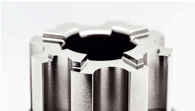
Stamping tool after processing
