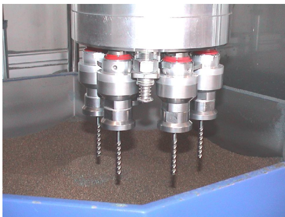
Fig.: Tool holder with workpieces just before immersion in the process container.
