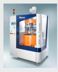
The DF-5 Tools drag finishing unit now has a brand new look. Of course, it is not only a matter of appearance. The welded, very rigid steel frame gives the machine an extremely compact chassis which enables larger and heavier workpieces (up to about 15 kg) to be finished in it. This once again opens up new opportunities for using the drag finishing process for the edge rounding, deburring, smoothing and polishing of tools.
