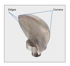
require surface finishing before they can be used in an aircraft or for power generation, since either the initial roughness is too great or the edges are too sharp. There are two tasks involved here:
