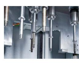
This made it clear that the DF 5 Standard would be used as a basis and that it would need to be equipped with a lot more space and much more power. The existing standard machine was redesigned to enable it to accommodate up to five workpiece holders with a minimum circumscribed circle of max. 330 mm.
