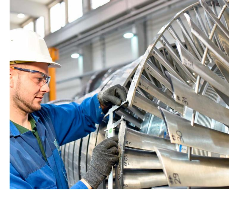
The manufacture of turbine blades involves many different mechanical manufacturing pro-cesses. These include forging, milling, casting and increasingly also additive manufacturing processes such as 3D printing in laser sintering. Simply milling a single turbine blade on a five-axis machine takes at least about an hour. After manufacturing, all parts
