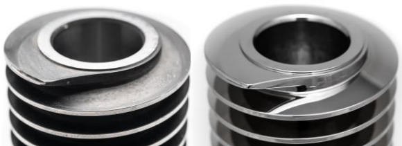
Extruder screw before (left) and after (right) processing with OTEC stream finishing
