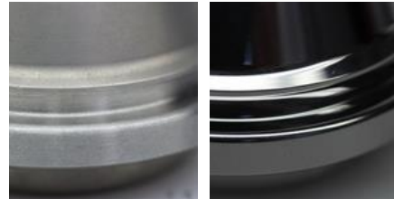
Seaming roll 0.44 \mu\text{m} before (left) and 0.05 \mu\text{m} after (right) processing with OTEC stream finishing
