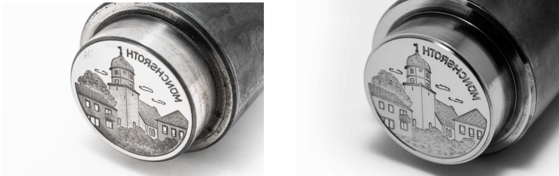
Coin hubs: example before (left) and after (right) processing with OTEC Dragfinish
