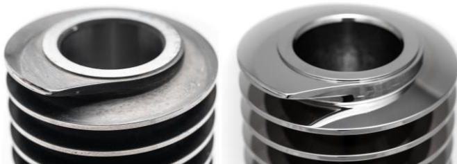
Extruder screw before processing with OTEC stream finishing
