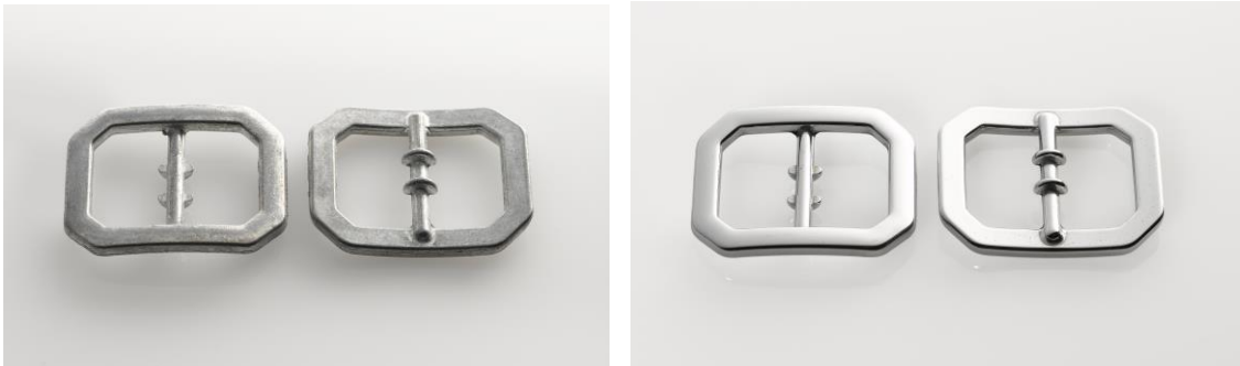
Belt buckle before and after processing in an OTEC disc finishing machine
