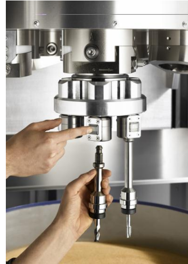
Changing the workpiece in the independently rotating holder
