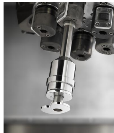
Angled, independently rotating workpiece holder with tibia
