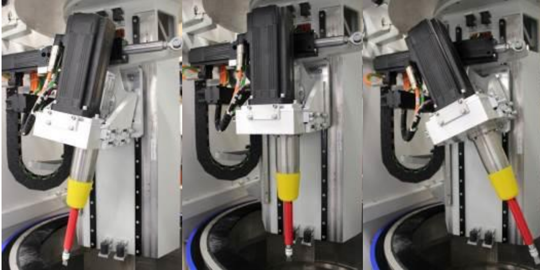
Fig. 3: The angle of incidence can be adjusted by means of a servo motor
