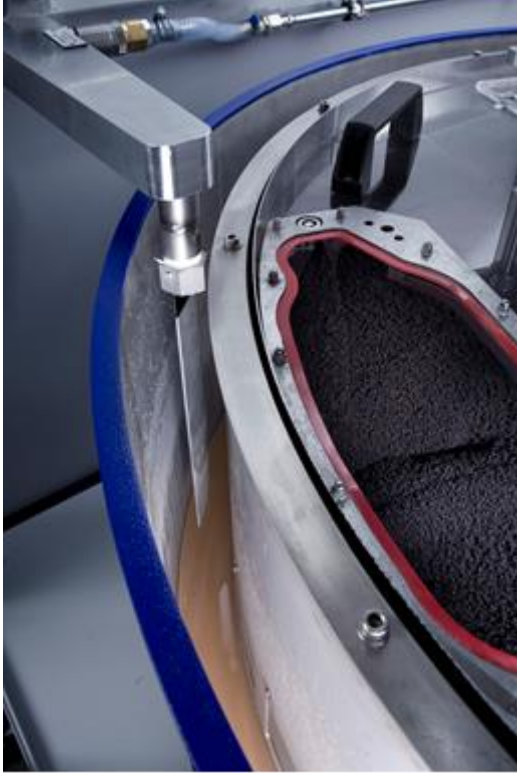
Fig. 4: Suction nozzle for extracting the waste water
