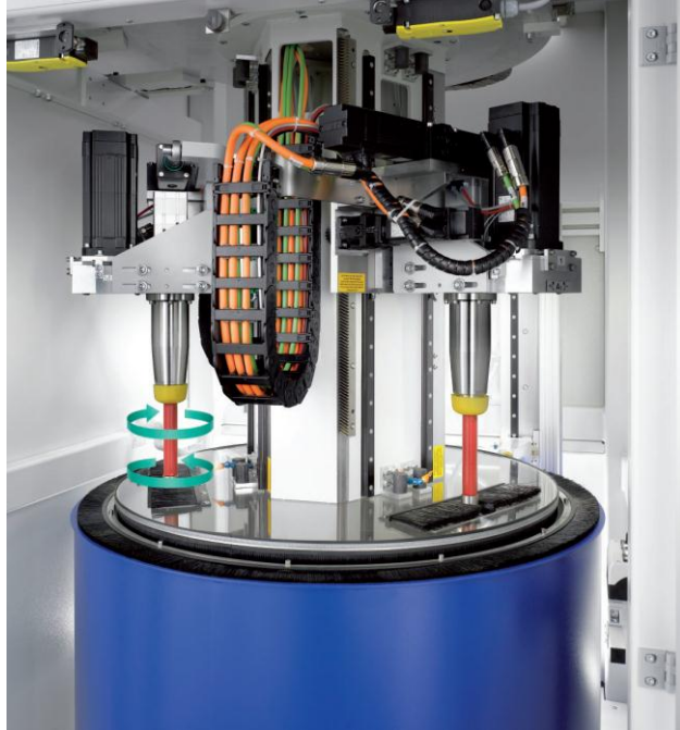
The oscillating spindle is accelerated to 2,000 rpm and decelerated again every second
